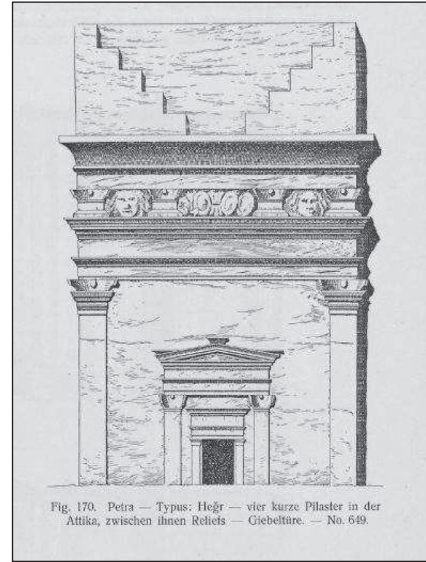
4. The Tomb No 649 with Double entablature (Brünnow and von Domaszewski I. 1904, fig. 170).
